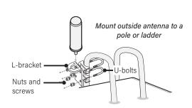
Mount the antenna to a pole or ladder. Position it upright position such that the entire length of the antenna is above the roof line of the RV and other metal obstructions.
