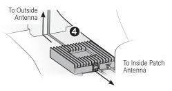
Select a well-ventilated location for the booster that is away from excessive heat, direct sunlight, and moisture. Beneath a seat or within the front console is suggested.
