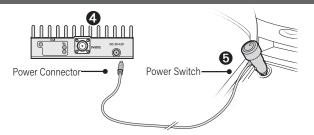
Connect the DC power cord connector to the signal booster and the adapter end to the cigarette lighter adapter to your vehicle. Once all connections are connected, turn the power switch on the adapter to ON. The POWER LED will briefly flash YELLOW/RED during initialization to indicate that the signal booster is ready for use.
