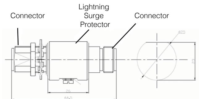
To ground your surge protector, use 10 or 12-gauge copper wire and attach it to the ground connector screw. Tighten the screw so the wire is firmly embedded under the screw. Next, clip the other end of the wire and strip back the jacket to expose the raw wire. Then, attach the wire to a grounding point or rod sunk into the ground 8 feet deep. Be sure to check your local grounding code requirements as they vary by location.
